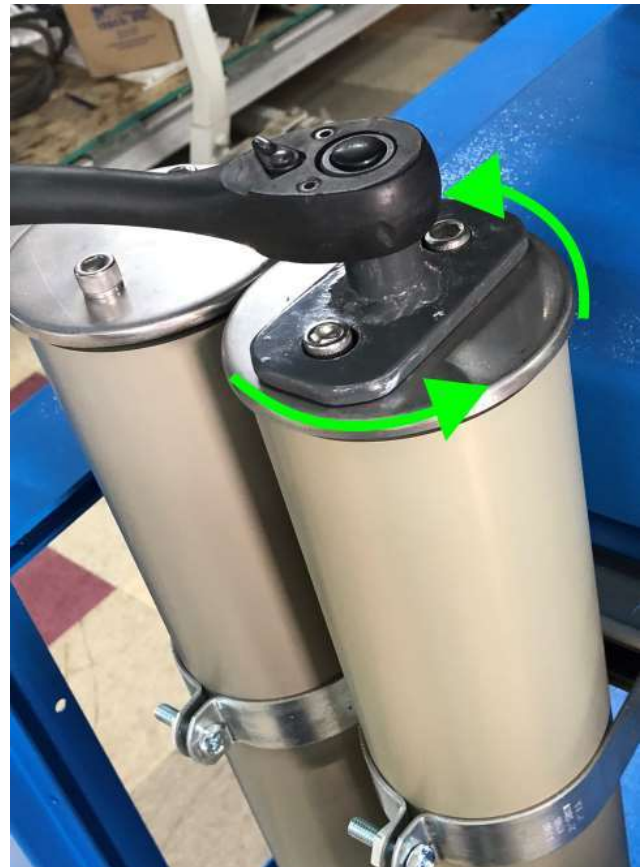
Figure 6.6: Cap Removal with Filter Wrench
