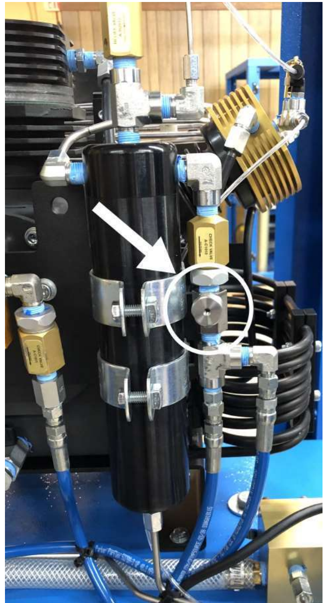
Figure 6.4: A1000/1060 Series Bleed Valve
