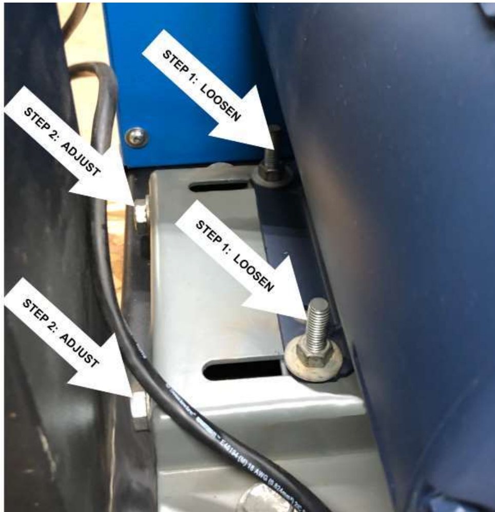
Figure 6.10: Open Frame Belt Tension Bolts
