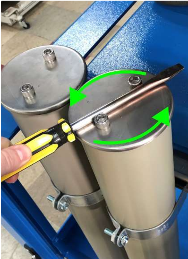
Figure 6.5: Cap removal with Screwdriver
