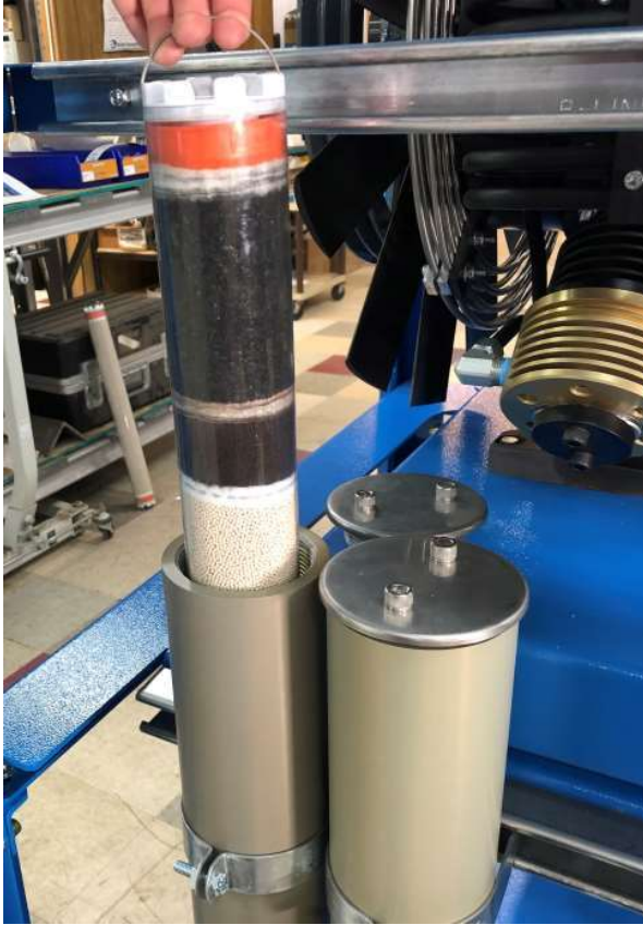
Figure 6.7 Filter cartridge removal.
